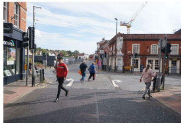
Example of crossing with both tactile information and dropped kerbs
