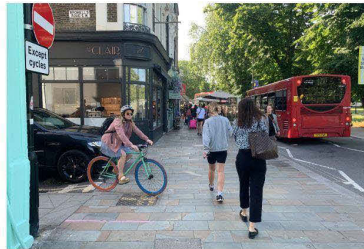
Continuous footway treatment further promotes pedestrian crossings
