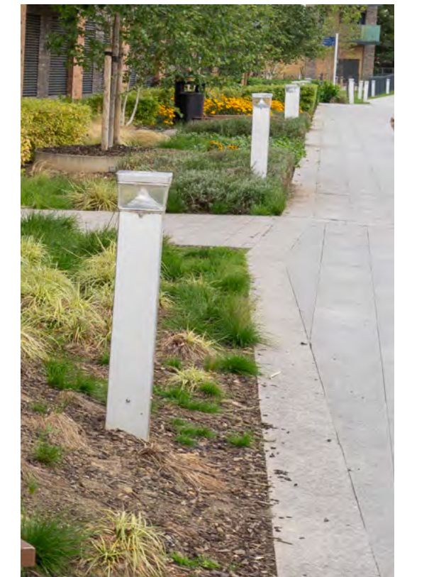
Figure 99. Stainless steel light bollards
