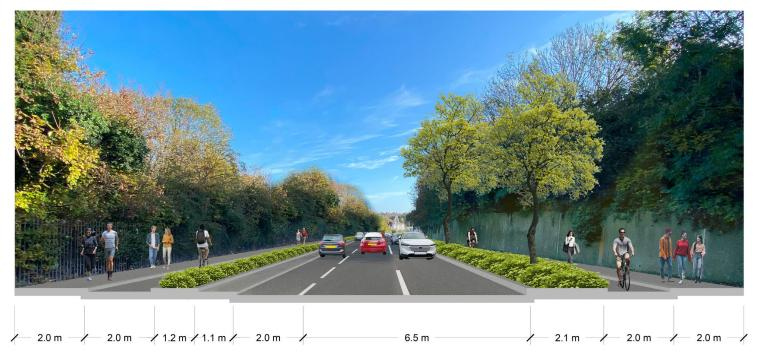
**Indicative cross section** as proposed at the stretch of London Road near Sandpiper Close. It shows the segregated cycle lane and walkway, each at 2 metres wide in each direction. On the left hand side (north) there is also an indicative greening strip and a 2 metre parking bay with a 1.1 metre wide pavement to allow for safe access to the vehicles.
